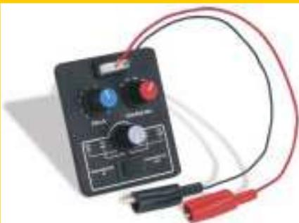
A truly universal adapter for NiCd and NiMH batteries only. All one has to do is connect the "UNIVERSAL ADAPTER" as though it was a typical battery cup. There are three rotary switches and a molex connector mounted on it.
